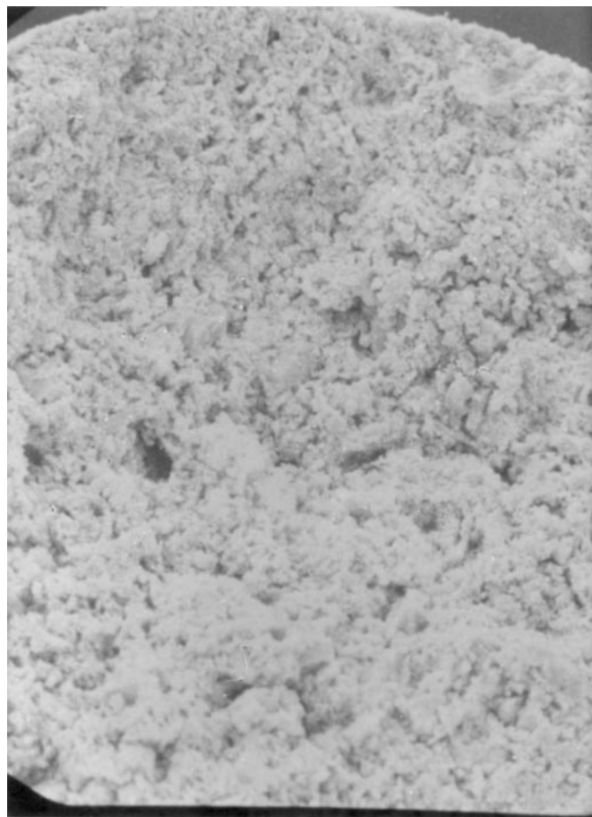
FIG. 16. 100 \mu\text{m} . Micrograph of the SiC support which shows the preservation of the extrudate shape.
