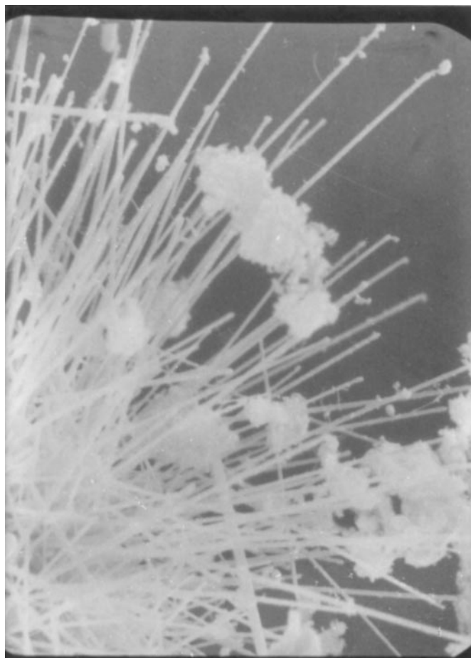
FIG. 6. 15 \mu\text{m} . Excessive whisker growth at the exterior of an extrudate, \text{H}_2/\text{SiCl}_4 = 26 ; T , 1380 K; P , 8 kPa; t , 3600 s.
